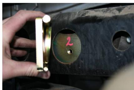
Position the No. 1 plate (LARGE WELDING ON SPACER BAR TO THE TOP) with the depressed centre into the hole in the chassis which is the first hole from the bend in the chassis.
